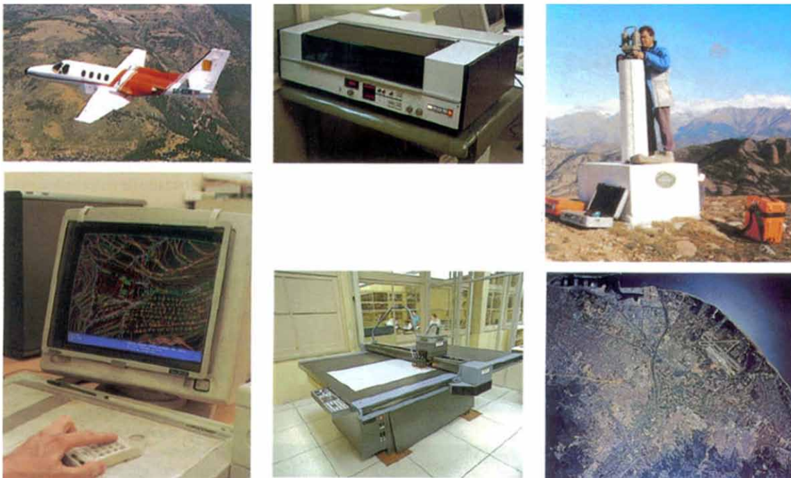
Figure 1. A classical group of figures of the 90s for the obtainment of analogical and digital images for digital cartography: plane with Wild RC-10 photogrammetric cameras, cameras for oblique photography Rollei 6008, etc.), scanner to digitalize analogical images, manual edition, plotter printer, etc., to get a high-resolution map, field work (geodesy)
