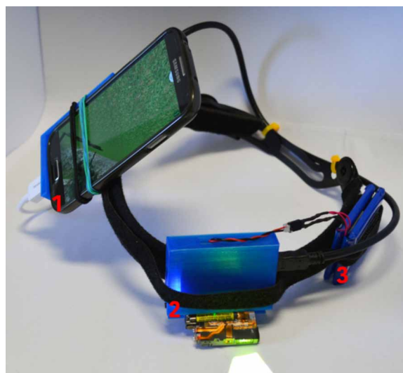
Figure 3. Picture of our HMPD consisting of (1) smartphone, (2) laser projector and (3) battery pack. As smartphone, we use a Samsung Galaxy S4+ that runs an app created in Unity 4, which processes the sensor data from the smartphone’s inbuilt gyroscope detecting head movements and holds the digital environments. The created digital environments are explained in more detail in a later section.
